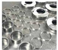
Laser cutting 2 Individual pressings for the end caps are laser cut. They're welded on the inside before the outside is polished.
