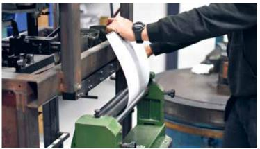
**Rolled and welded** At the start of the production process all exhausts begin as a flat blank that is rolled into the desired shape (either round or oval), tacked and then seam-welded.
