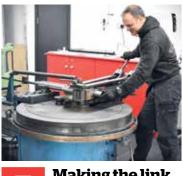
**Making the link** 5 Link pipes are formed on the pipe bender and if necessary reduced on the swaging machine.
